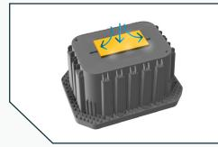
Tier 12 testing uses a larger 10" x 20" steel plate (illustrated in yellow) to apply the 33,750 lb. load from the hydraulic press, simulating a wheelbase of a heavy truck interacting with the enclosure, and dispuring the load more evenly accross the cover.
