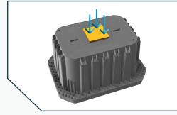
Tier 15 testing uses a 10" x 10" steel plate (illustrated in yellow) to apply the 22,500 lb. load from the hydraulic press, simulating the wheelbase of a passenger vehicle interacting with the enclosure.
